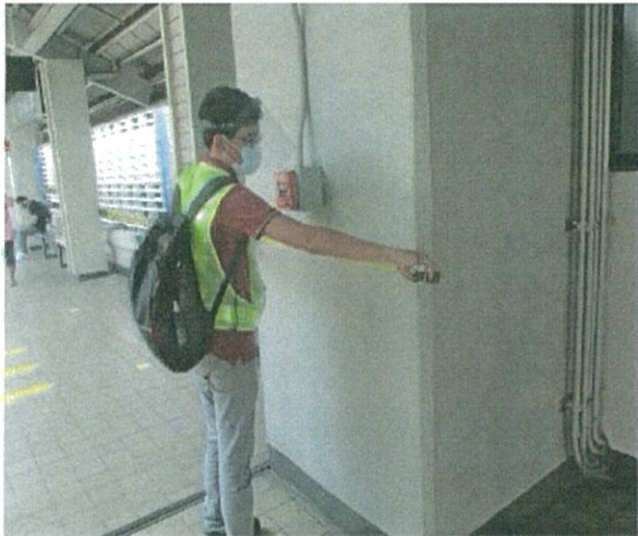
VERIFICATION OF COLUMN DIMENSIONS AT CARRIEDO STATION
