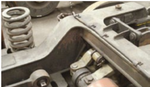
Bogie frames that need replacement
