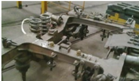
Bogie frames that need replacement
